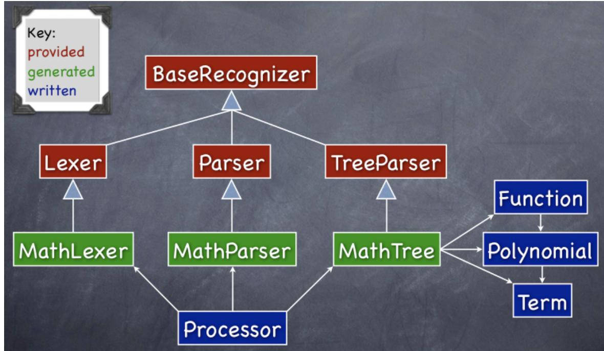
Note the key in the upper-left corner of the diagram that distinguishes between classes provided by ANTLR, classes generated from our grammar by ANTLR, and classes we wrote manually.
