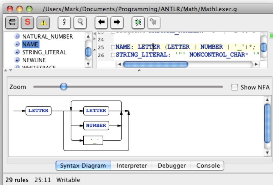
Here's an example of a syntax diagram for a selected parser rule.
